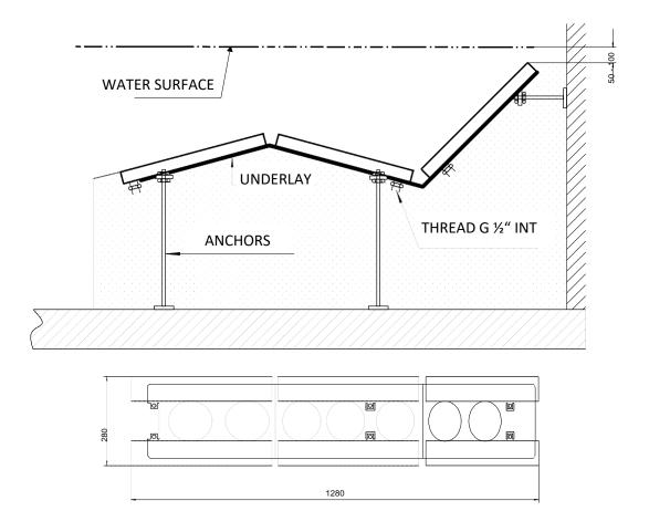
The massage seat itself is made of AISI 304 stainless steel (NOT SUITABLE FOR SALTWATER POOLS), the remaining parts of galvanized steel. The stainless-steel part is pickled and polished, with the flange bolts in A4 material. In liner pools, the seat flange is sealed only with the liner.
